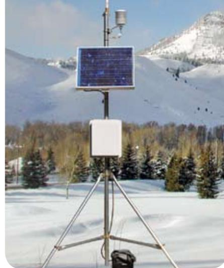
▲ Solar Powered Weather Station
