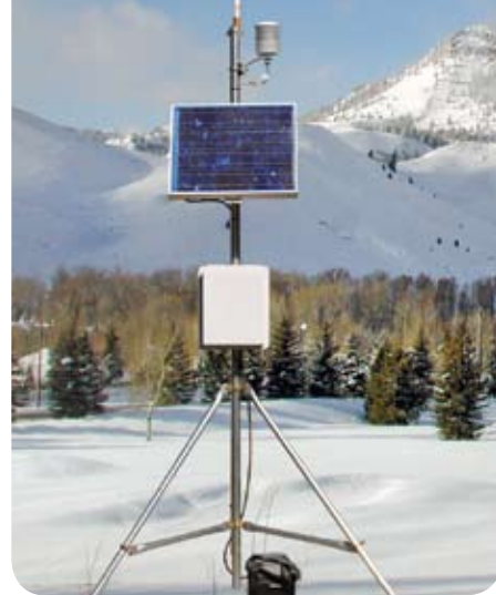
▲ Solar Powered Weather Station
